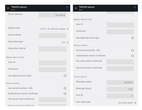
TN5250 is a variation of the Telnet protocol and is used by the IBM5250 emulation to connect to IBM hosts over a TCP/IP network. You can either connect directly to the host if it's running a Telnet server, or via a TN5250 gateway.
