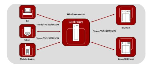
The GlinkProxy application runs on a Windows server that can be located near the host computer. It will allow the traffic from the mobile computers, tablets or PCs with Glink to be routed through the GlinkProxy server to the host. The GlinkProxy server will keep the connection to the host application even if the connection to the client computers with Glink is lost. When Glink reconnects, the session with the host application will resume as if the connection was not lost.
