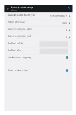
Glink can either receive scanner data as simulated keyboard input (Keyboard Wedge) or receive scanner data through device specific configuration. Most scanners are using Keyboard Wedge by default.
