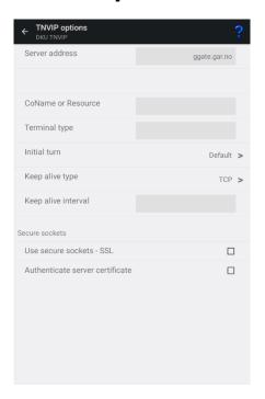
TNVIP is a variation on the Telnet protocol and is used by Bull synchronous emulations to connect to Bull hosts via a TNVIP gateway over a TCP/IP network.
