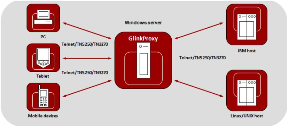
The GlinkProxy application runs on a Windows server that can be located near the host computer. It will allow the traffic from the mobile computers, tablets or PCs with Glink to be routed through the GlinkProxy server to the host. The GlinkProxy server will keep the connection to the host application even if the connection to the client computers with Glink is lost. When Glink reconnects, the session with the host application will resume as if the connection was not lost.
