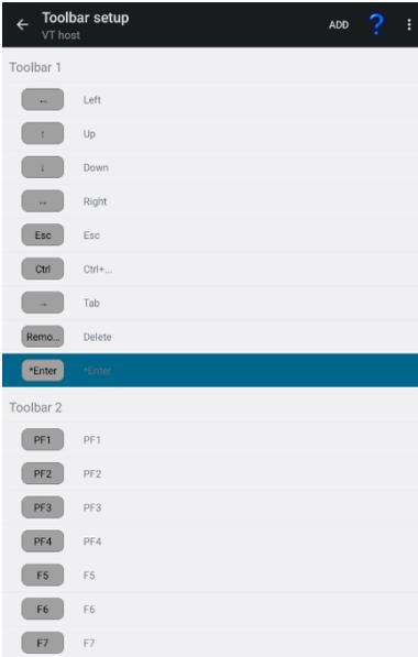
For the *Screen options* -> *Show toolbar* values: *Auto*, *Multiline* and *Single-line* the toolbars will be displayed horizontally with *Toolbar 1* as the first toolbar row, *Toolbar 2* as the second toolbar row and so on.
