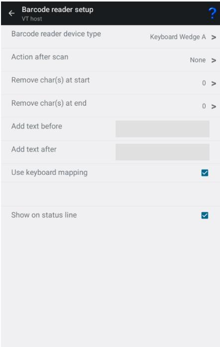
Glink can either receive scanner data as simulated keyboard input (Keyboard Wedge) or receive scanner data through device specific configuration. Most scanners are using Keyboard Wedge by default.
