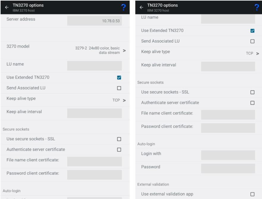
TN3270 is a variation on the Telnet protocol and is used by the IBM3270 emulation to connect to IBM hosts over a TCP/IP network. You can either connect directly to the host, if it's running a Telnet server, or via a TN3270 gateway.
