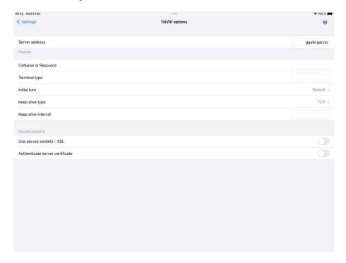
TNVIP is a variation on the Telnet protocol and is used by Bull synchronous emulations to connect to Bull hosts via a TNVIP gateway over a TCP/IP network.
