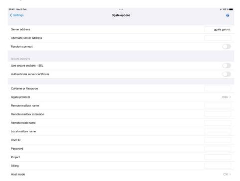
Ggate is a gateway product available from G&R for UNIX and Windows platforms. It allows Glink to connect over TCP/IP to Bull and IBM hosts which use the ISO/DSA protocol for network communications.
