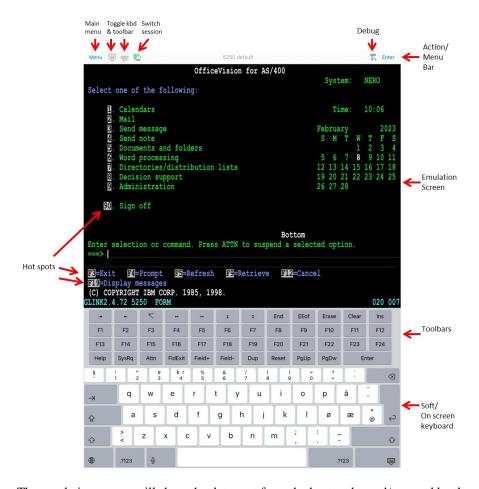
The emulation screen will show the data sent from the host and typed/scanned by the user. In **Menu -> Settings -> Screen options** you can customize the look of the emulation screen. The most important options are the *Font size*, *Show toolbar*, *Limit screen view* (x,y) and the options for *Hotspots*.
