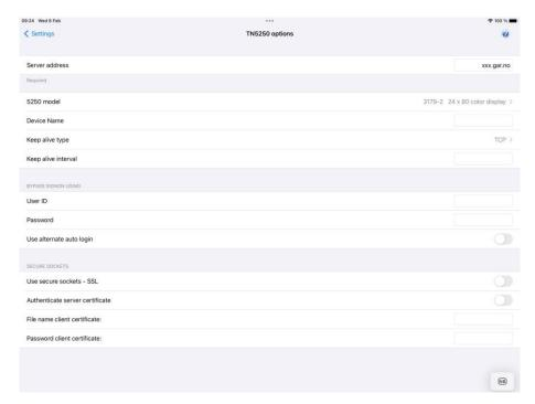
TN5250 is a variation of the Telnet protocol and is used by the IBM5250 emulation to connect to IBM hosts over a TCP/IP network. You can either connect directly to the host if it's running a Telnet server, or via a TN5250 gateway.
